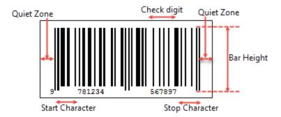
**Bar Height**: Enter a value in inches (for example, .25in) for the height of the barcode.
