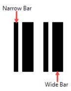
**Tip**: For accurate scanning, the quiet zone should be ten times the Narrow Bar Width value.
